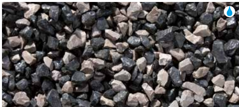
Basalt chips, Black and Limestone chips, Mouse grey, 8–12 mm
