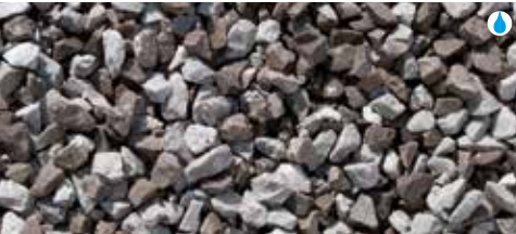
Marble chips, Silver grey and Limestone chips, Mouse grey, 9–12 mm
